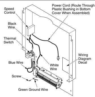
Figure 18 - Blower Wiring Layout (Thermostat Blower Shown)
